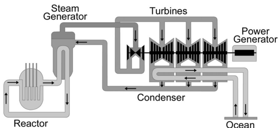
**Fig. 1.** Schematic view of the cooling system of CNAAA.
