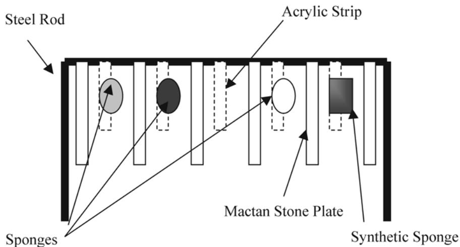
**Fig. 1.** Mactan stone settlement plate rack with treatment sponges, synthetic sponge control and acrylic strip control.
