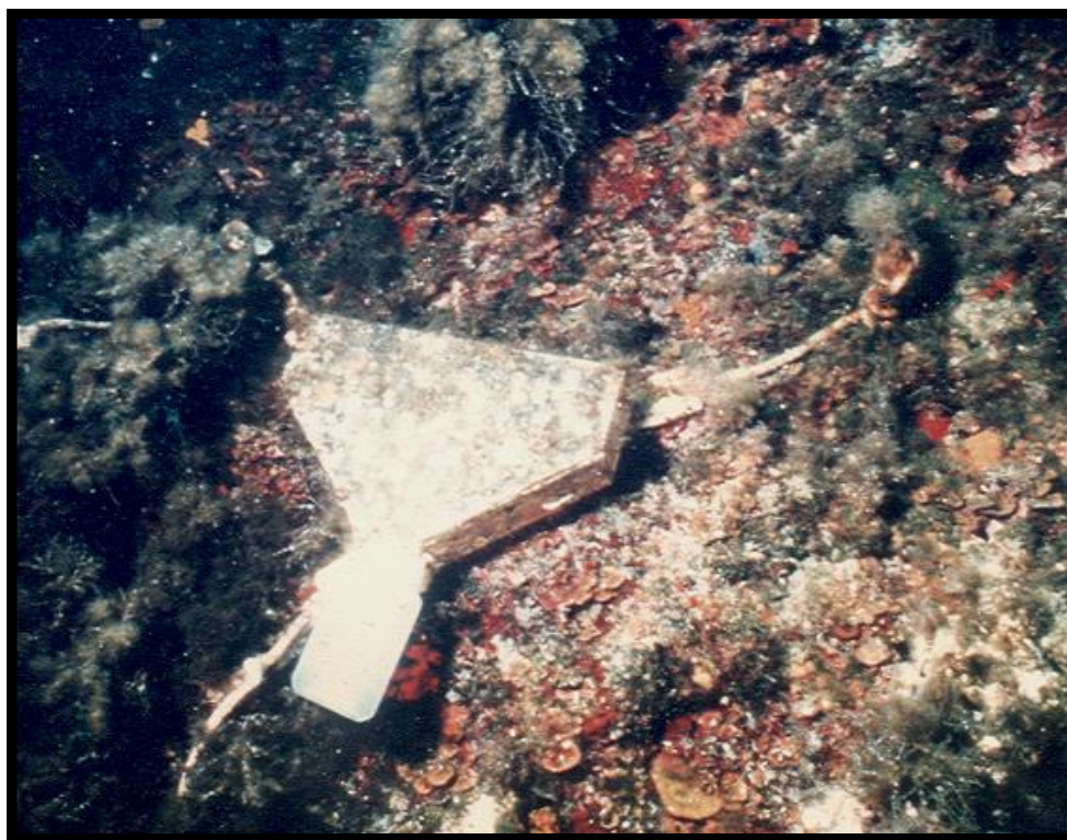
Figure 8. A trap to collect sediments rolling down the cliff.
