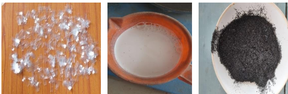
Figure 2. Additives used for the test: plastic strips, rubber latex, coir fiber ash.
